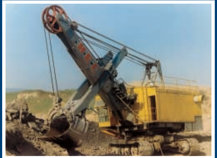
Electric Rope Shovel, 5 Cu. M.
