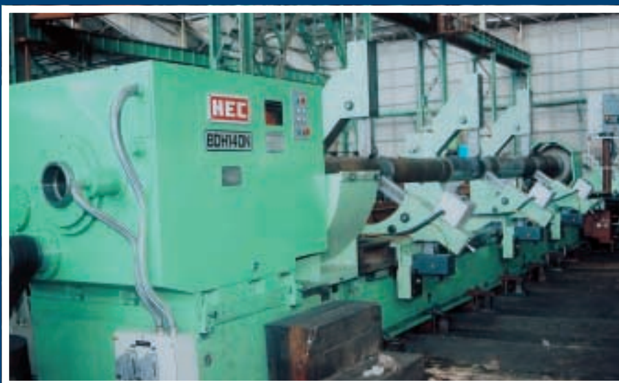
CNC Deep Hole Boring Machine for M.S.F. Ishapore
